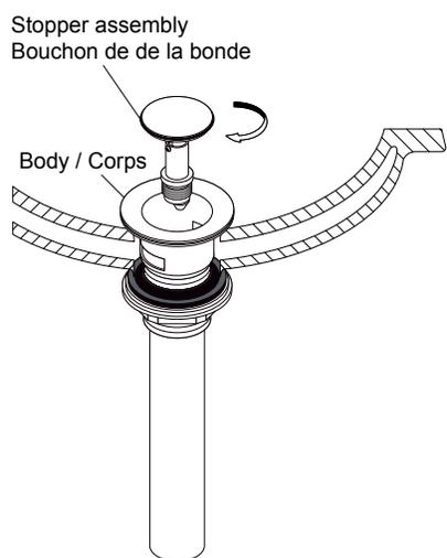
3. Put stopper assembly into drain.
