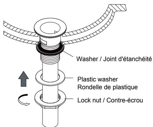
2. Install washer, plastic washer and lock nut onto pop-up body from underneath the basin.
