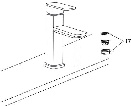
3. Remove aerator(17) and open the hot and cold water supplies.
