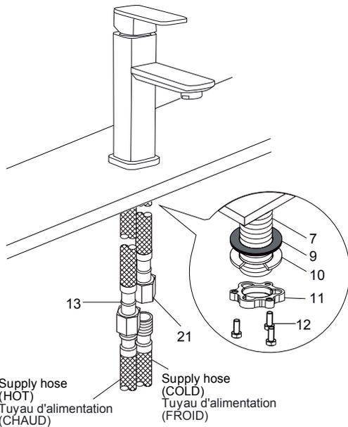
2. Screw lock nut(11), metal washer(10) and rubber washer(9) onto the pipe(7) by screws(12).
