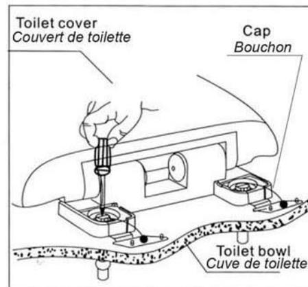
1. Place the toilet seat cover on bowl, insert the bolt, washer and rubber cord in hinge install hole-order;
