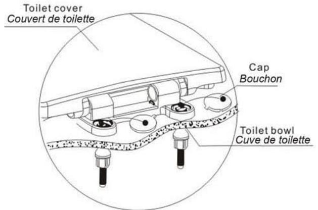
2. Insert the nut into the two holes perfectly and screw it with screwdriver, then put the cap on it.
