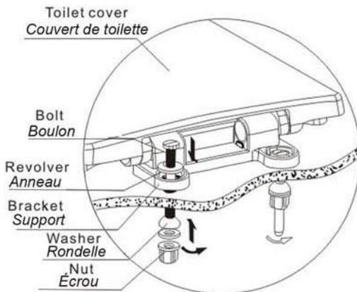
1. Insert revolver, washer and bolt into the installing hole.
