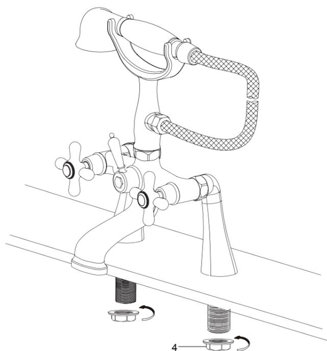
4. Tighten nut(4) onto the water way.
