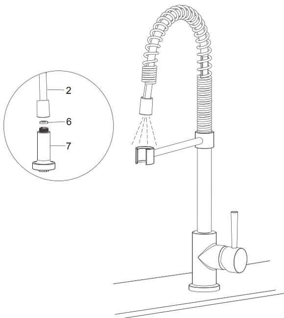
4. Open the hot and cold water supplies. Check for leaks. Turn on the faucet handle for one minute to flush debris from faucet. Close the handle and re-assemble the spray(7) on the hose(2).
