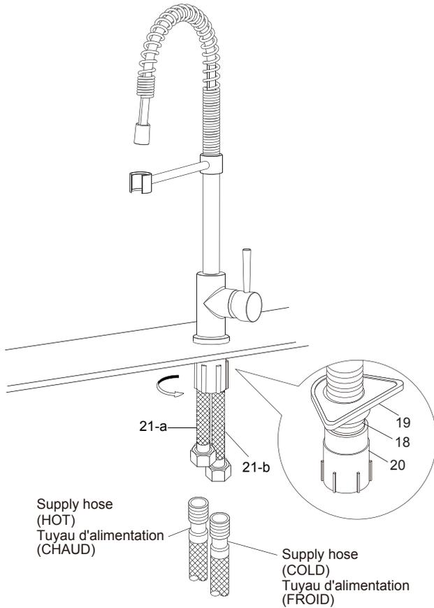
3. Tighten mounting nut(20) and plastic washer(19) onto the pipe(18). Screw the supply hose(not included) on the hot hose(21-a) and cold hose(21-b).
