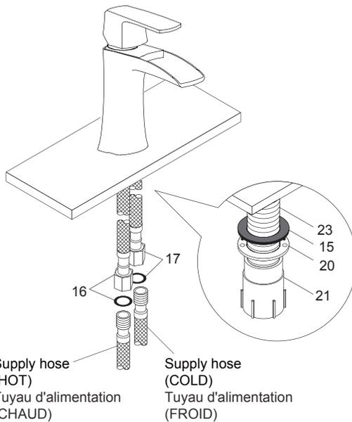
2. Screw lock nut(21), metal washer(20) and rubber washer(15) onto the pipe(23).
