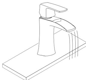
3. Check for leaks. Turn on faucet handle for one minute to flush debris from faucet.
