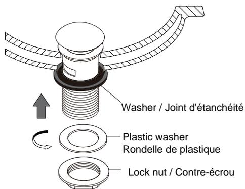
2. Install washer, plastic washer and lock nut onto pop-up body from underneath the basin.
