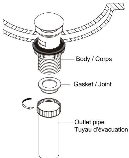
3. Screw outlet pipe on the body.
