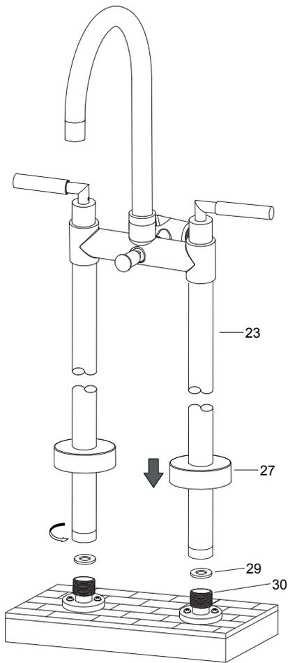
3. Connect the water way(23) and the rubber washer(29) with the shank(30).
