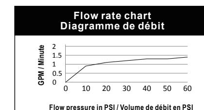
Because of difference of city water system or others, water pressure may differ, and cause the flow rate to change a little bit.
