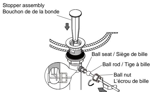
2. Put stopper assembly into drain.
