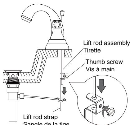
4. Insert bottom of lift rod assembly into hole at top of lift rod strap. Tighten with thumb screw.
