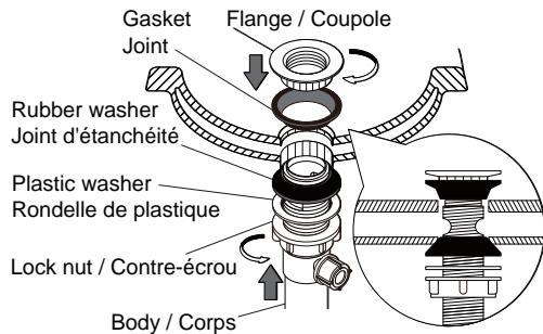
1. Install plastic washer, rubber washer and lock nut onto pop-up body from basin underneath.
