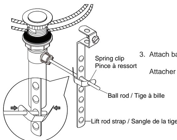
3. Attach ball rod to lift rod strap using spring clip.
