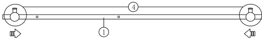
Position the stoppers(4) on the running rail (1) as illustrated. Secure them temporarily in place.
