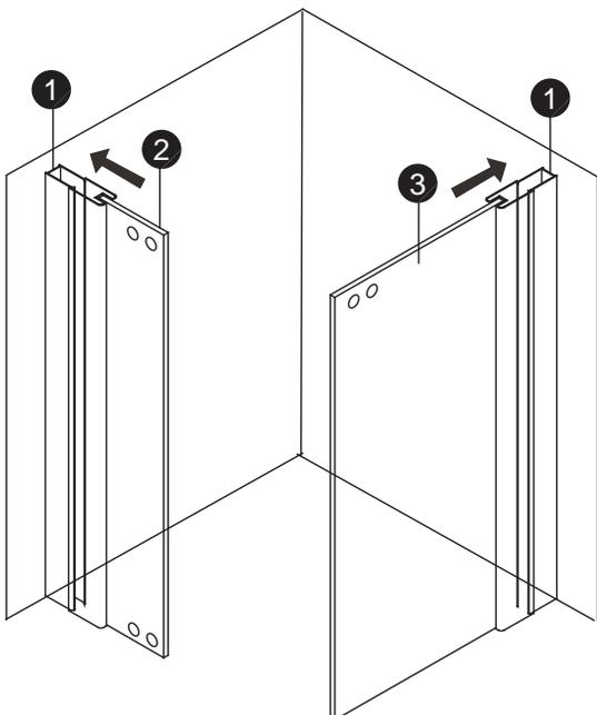
Slide the fixed panel (2) and the fixed side panel (3) into the wall jambs (1).
