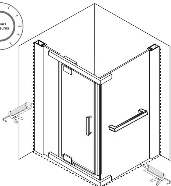
Apply silicone sealer around all external joints of shower door and allow 24 hours for silicone to set. Silicone is not used on the inside of the shower screen because in time water can build up with in the wall jamb and cause leaks outside of the shower area. The screens are designed to allow the water to return into the shower area, if needed.
