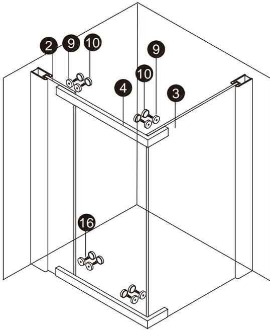
Connect top and bottom rails (4) to fixed panels (2) and (3). Ensure rail cap bases (9) are placed on the glass before using rail fixing screws (16). Cap off with rail caps (10). Do not over tighten as this may damage rail cap bases (9).
