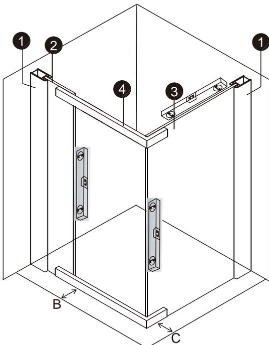
Adjust fixed panels (2) and (3) in or out of the wall jambs (1) so that the top rail (4) is horizontal and the whole panel sits level on the shower base / shower area. (Bmm = Cmm). Also, make sure both fixed panels (2) & (3) sit vertically.
