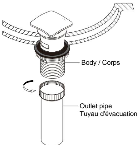
3. Screw outlet pipe on the body.
