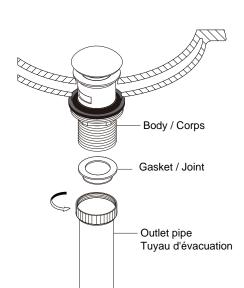
3. Screw outlet pipe on the body.
