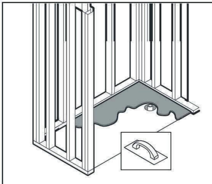
**Step: 4.** Make sure all the legs of the tub are entirely touch the floor. If not, adjust them or set the level or use a mortar bed for proper installation.
