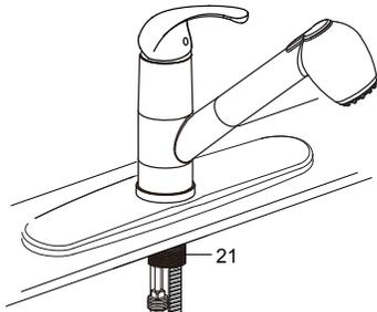
2. Tighten mounting nut(23) and plastic washer(26) onto the pipe(21).
