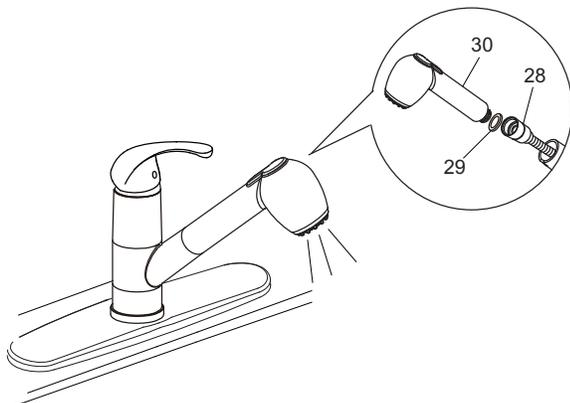
4. Open the hot and cold water supplies. Check for leaks. Turn on the faucet handle for one minute to flush debris from faucet. Close the handle and re-assemble the spray(30) on the hose(28).
