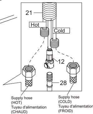
3. Connect hose(28) with quick connector(12). Assemble weight and screws(27) on the hose(28). Screw the supply hose(not included) on the hot inlet pipe and cold inlet pipe.
