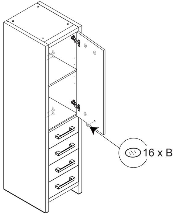
The linen cabinet wall mounting screws need to be fixed onto the studs behind the dry wall board. Locate and mark the stud positions with a stud finder and drill pilot mounting holes at marks onto the desired studs. Insert the plastic screw sleeves into the drilled mounting holes on the wall. Drill the screw holes in the linen cabinet back panel to match the mounting holes on wall. Install the mounting screws through the linen cabinet back panel and dry wall board into the studs.
