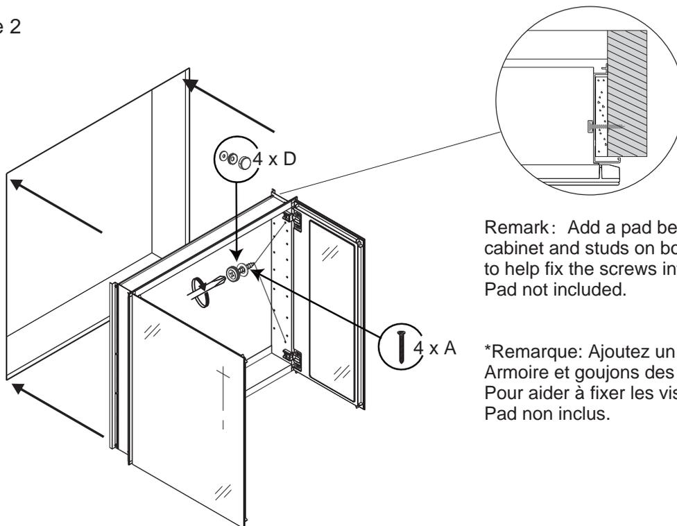
Remark: Add a pad between cabinet and studs on both sides to help fix the screws into the studs. Pad not included.
