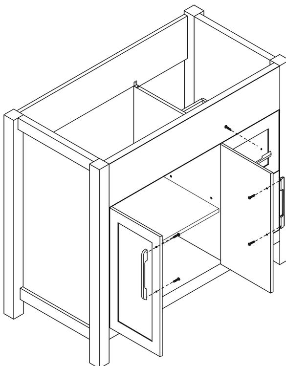
The vanity wall mounting screws need to be fixed onto the studs behind the dry wall board. Locate and mark the stud positions with a stud finder, drill pilot mounting holes at marks onto desired studs. Insert the plastic screw sleeves into drilled mounting holes on the wall. Drill the screw holes on vanity back panel to match the mounting screws through the vanity back panel and dry wall board to the studs.
