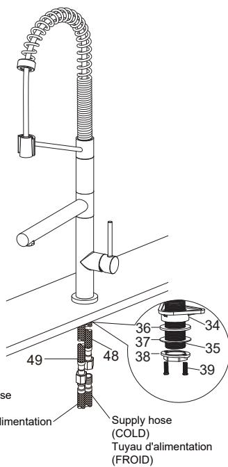
2. Place in order: the plastic washer(34), the rubber washer(36), the metal washer(37) and screws(39) on the pipe(35).
