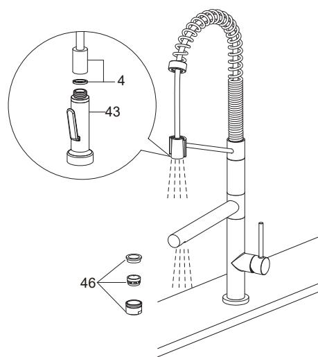
3. Remove aerator(46) and open the hot and cold water supplies.
