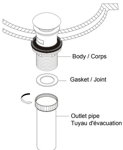
3. Screw outlet pipe on the body.
