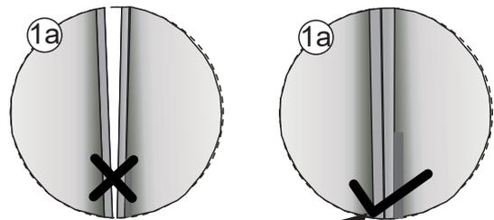
⚠ Adjust the sliding doors using the screws located on the bottom of top roller assemblies. Adjust rollers so that the sliding doors are parallel to the fixed panels and parallel to each other.
