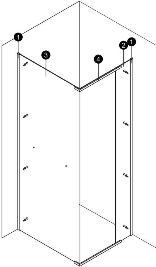
Now drill 4 equally spaced 3.2mm holes into the wall jamba (1) on the **INSIDE** of the screen. Make sure that your drill holes are more than 30mm away from the edge of the glass, when using smallest screen size, otherwise you may break the glass. Make sure that the holes also go through the aluminium of the fixed panels. Fix the fixed panels (2) & (3) using the fixed panel screws (20) and caps (21).
