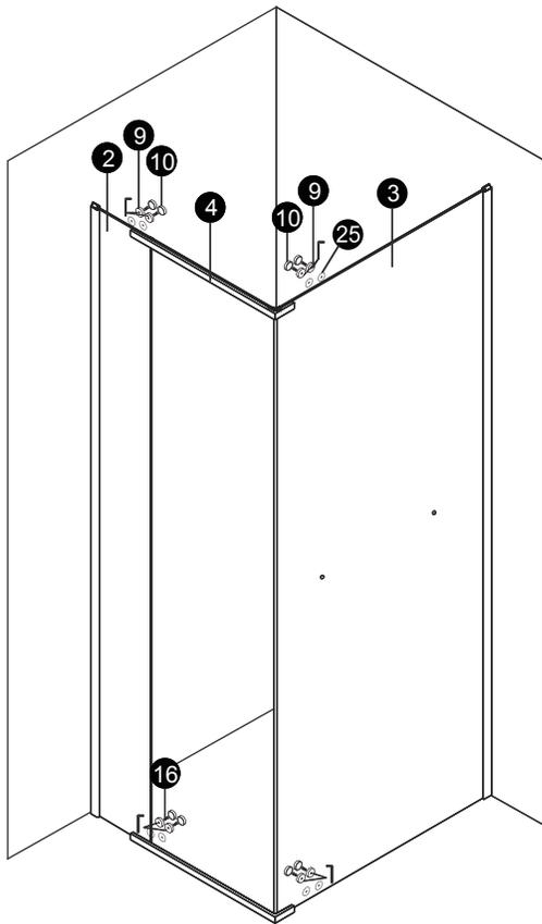
Connect top and bottom rails (4) to fixed panels (2) and (3). Ensure rail cap bases (9) are placed on the glass before using rail fixing screws (16). Cap off with rail caps (10). Do not over tighten as this may damage rail cap bases (9).
