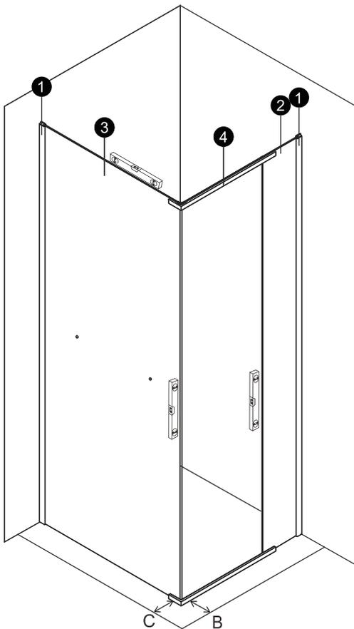
Adjust the fixed panel (2) and (3) in or out of the wall jambs (1) so that the top rail (4) is horizontal and the whole screen sits square on the shower base / shower area. (Bmm = Cmm). Also make sure both fixed panels (2) & (3) sit vertically.
