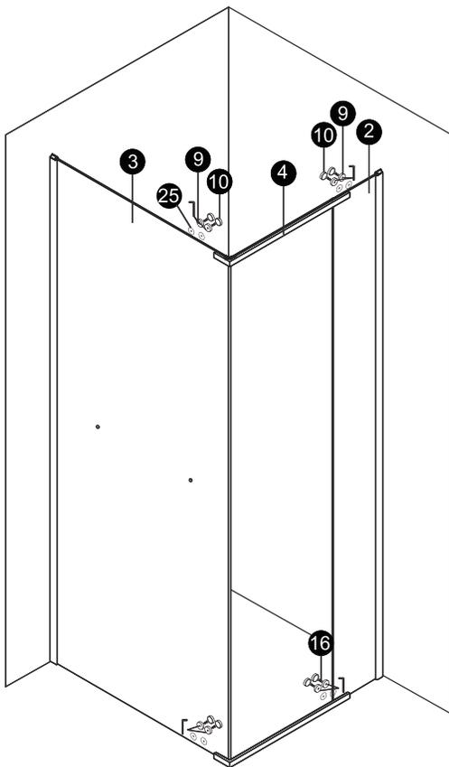
Connect top and bottom rails (4) to fixed panels (2) and (3). Ensure rail cap bases (9) are placed on the glass before using rail fixing screws (16). Cap off with rail caps (10). Do not over tighten as this may damage rail cap bases (9). Hint: Use a small amount of silicone on the cap to seal the cap to the cap base. Do this last when sealing the shower.
