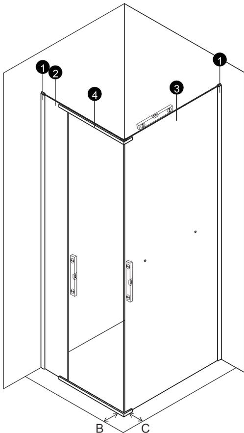
Adjust fixed panel (2) and (3) in or out of the wall jambs (1) so that the top rail (4) is horizontal and the whole screen sits square on the shower base / shower area. (Bmm = Cmm). Also make sure both fixed panels (2) & (3) sit vertically.
