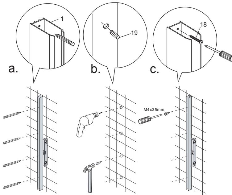
**The line mark is for reference only. Please mark according to your actual measurement. Make sure your measurements are correct and that they match the base and door before you drill the holes.**
