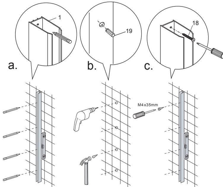
**The line mark is for reference only. Please mark according to your actual measurement. Make sure your measurements are correct and that they match the base and door before you drill the holes.**
