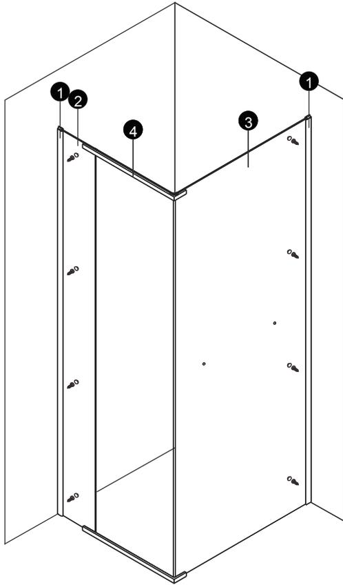
Now drill 4 equally spaced 3.2mm holes into the wall jamba (1) on the **INSIDE** of the screen. Make sure that your drill holes are more than 20mm back from the edge of the glass, when using smallest screen size, otherwise you may break the glass. Make sure that the holes also go through the aluminium of the fixed panels. Fix the fixed panels (2) & (3) using the fixed panel screws (20) and caps (21).
