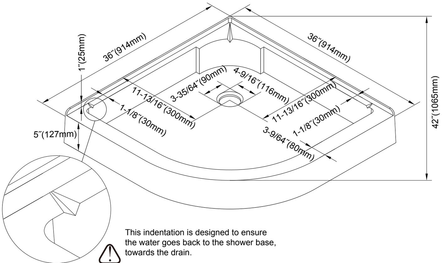
This indentation is designed to ensure the water goes back to the shower base, towards the drain.
