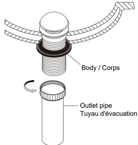
3. Screw outlet pipe on the body.
