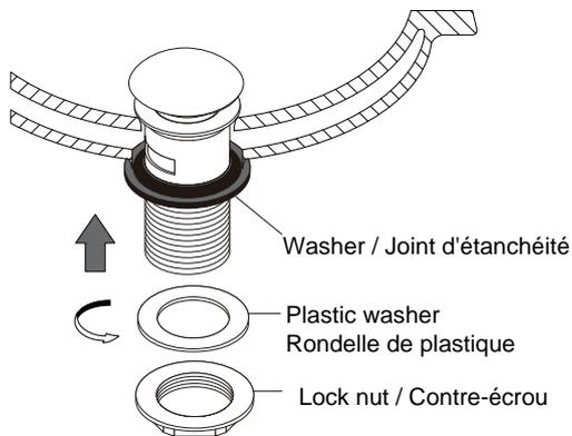
2. Install washer, plastic washer and lock nut onto pop-up body from underneath the basin. And then tighten lock nut.
