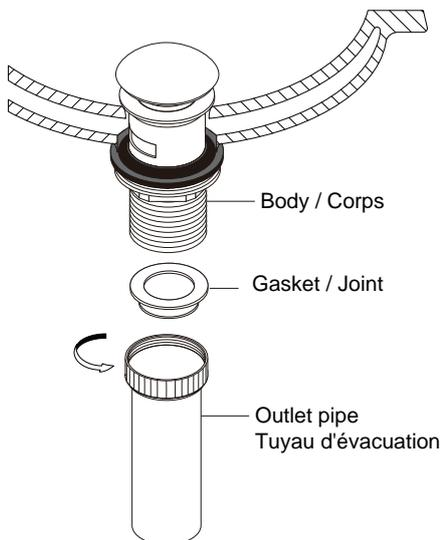
3. Screw outlet pipe on the body.
