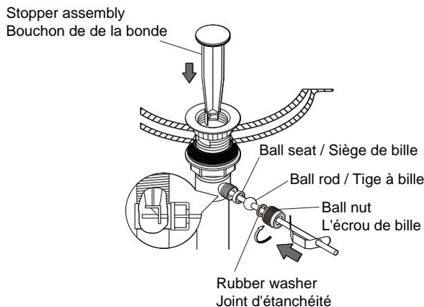
2. Put stopper assembly into drain.
